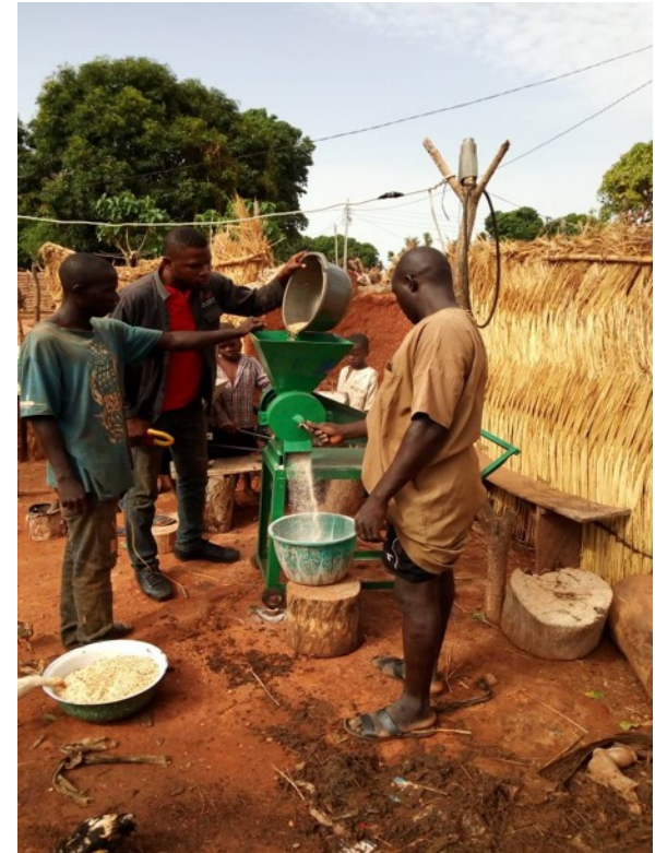
An operator-financed, electric-powered milling machine (Source: Nayo Technologies Ltd)
